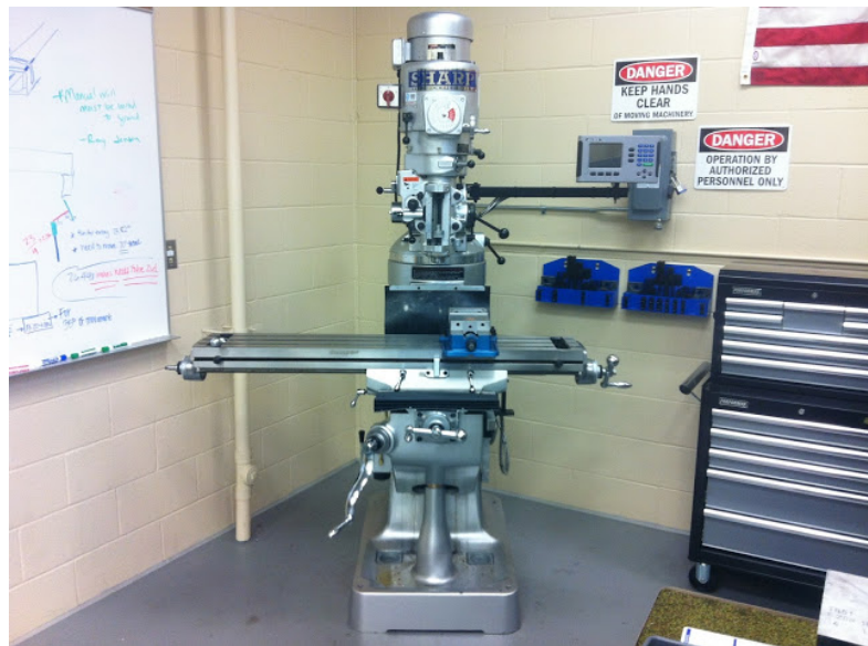
Manual Mill for training in machining, http://irengineering.blogspot.com/
